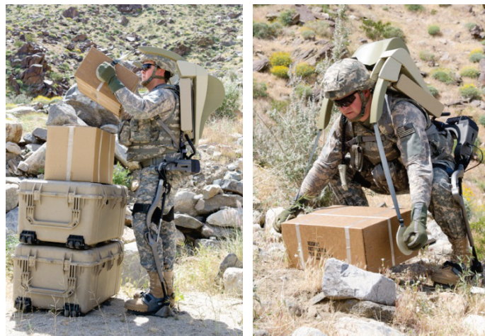
Figure 7.1. The HULC Exoskeleton by Lockheed Martin 45 .
