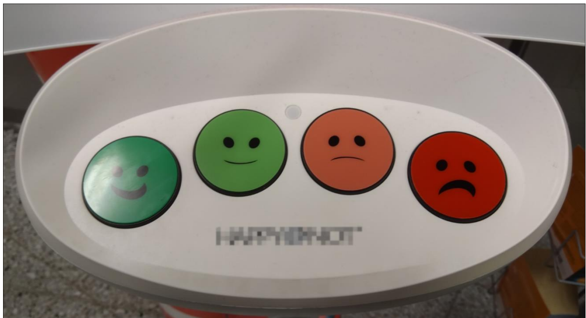
Figure 8 A customer feedback terminal from a retail store using pictographs for input. The terminal itself is a service provided by a third-party company. User feedback to an input is dim light at the top of the unit.
