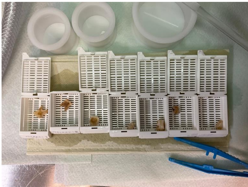
Figure 8. Infiltrated teeth and embedding moulds filled with the polymerisation solution
