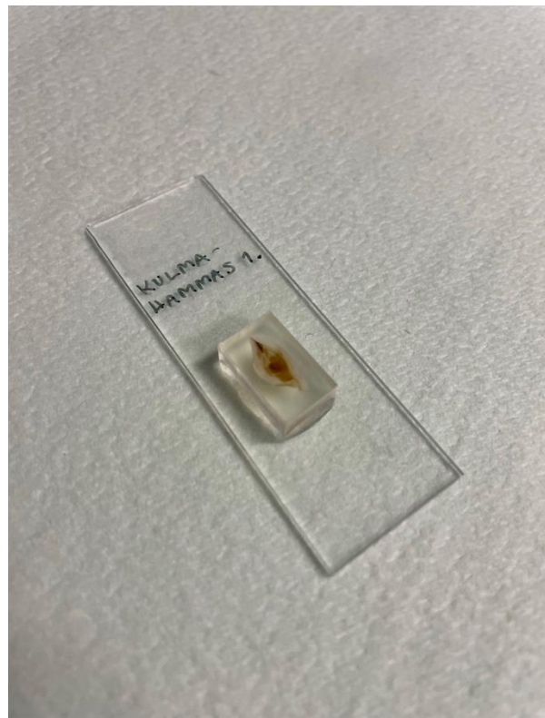
Figure 14. A completed block plexiglass
