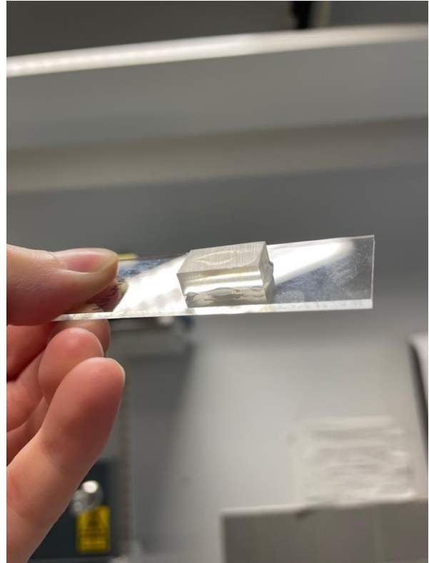
Figure 16. Confirming that the wanted specimen surface is exposed by examining it against light
