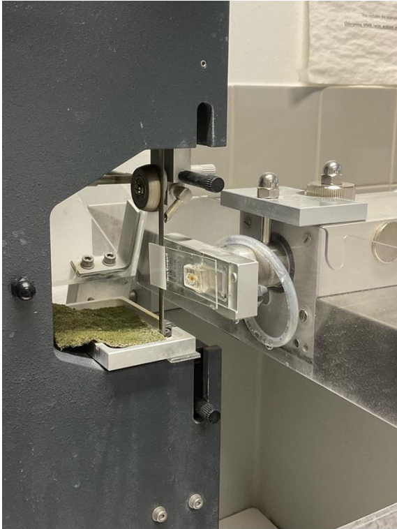
Figure 19. The specimen plexiglass was separated from the block by sawing
