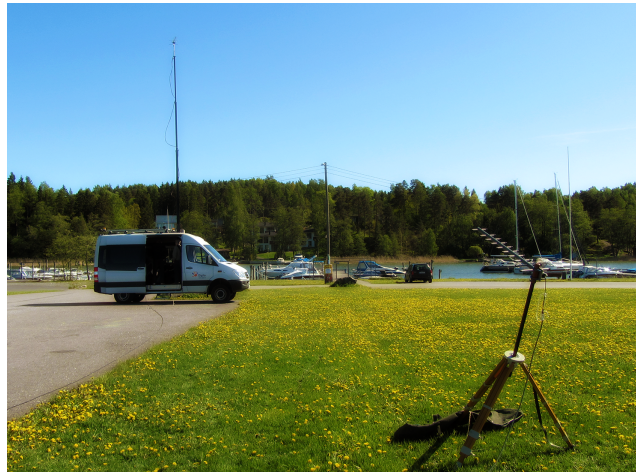
Figure 6: TVWS radio antenna at 1,5m above ground level (on the right) and 10m DTT reception antenna (on the left) in an outdoor reference geometry measurement.
