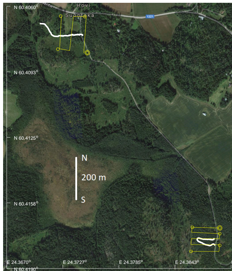
Figure 2. Trail 1 (below) and Trail 2 (above) are separated by approximately 1 km. The geo-reference markers are depicted by circles, the flight path is shown with the yellow cross-line and the trails by thick white curves. Trail 2 was not fully covered by the UAV photogrammetry. The starting points of the flight paths are indicated by the double circle.
