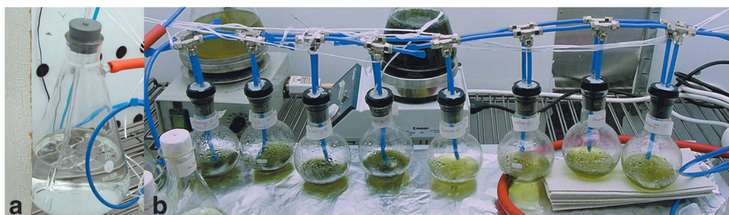
Figure 5: Vacuum line set-up where the gas flow is first saturated with water vapor (left) and then lead into the culture bottles. The gas flow is regulated with a rheostat and the pressure inside the closed system is controlled by a pressure gauge, and a vacuum pump
