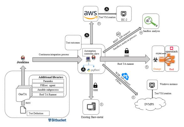
Figure 6: Actual system design and principal of workflow of the OneTA solution
