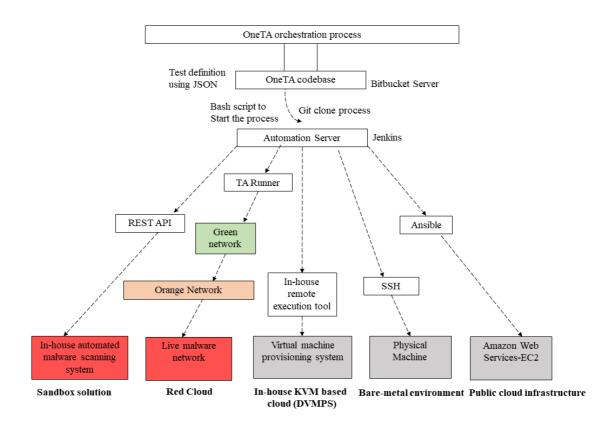
Figure 1: The principal of OneTA test orchestration solution
