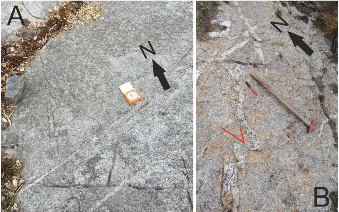
Fig. 44. A) Undeformed equigranular gabbro from near the NE margin of the intrusion. TALE-2017-17. N: 6771785, E: 274010. B) Heavily deformed gabbro where quartz has precipitated into dextral tension gashes, and is broken off into shorter segments by dextral faults (marked by a red half-arrow) that form a network with antithetic sinistral faults. TALE-2017-203. N: 6771840, E: 274025. The distance between the two observations is 60 m (see Fig. 39).
