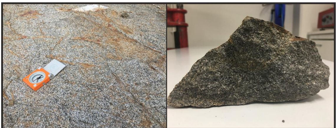
Fig. 13. Left: Deformed gabbro crosscut by rusted quartz veins. TALE-2017-203. N: 6771836, E: 274025. Right: Fresh surface of the gabbro in hand specimen.
