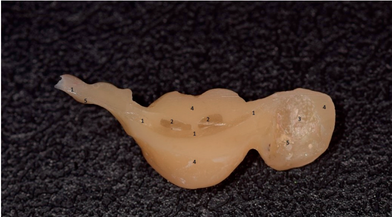
Figure 6. Longitudinal section of an FRC FDP showing the multiphase structure and location of the adhesive interphases. 1. Main continuous unidirectional FRC framework between abutments. 2. Continuous unidirectional FRC for pontic reinforcement. 3. Continuous multidirectional FRC for crown unit reinforcement. 4. PFC veneering composite. 5. Bonding site for resin cement.
