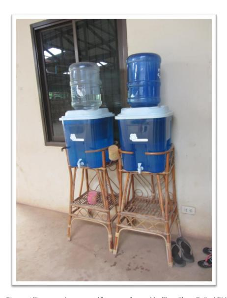
Picture 4 Two ceramic water purifiers manufactured by TerraClear, © Outi Pitkänen
