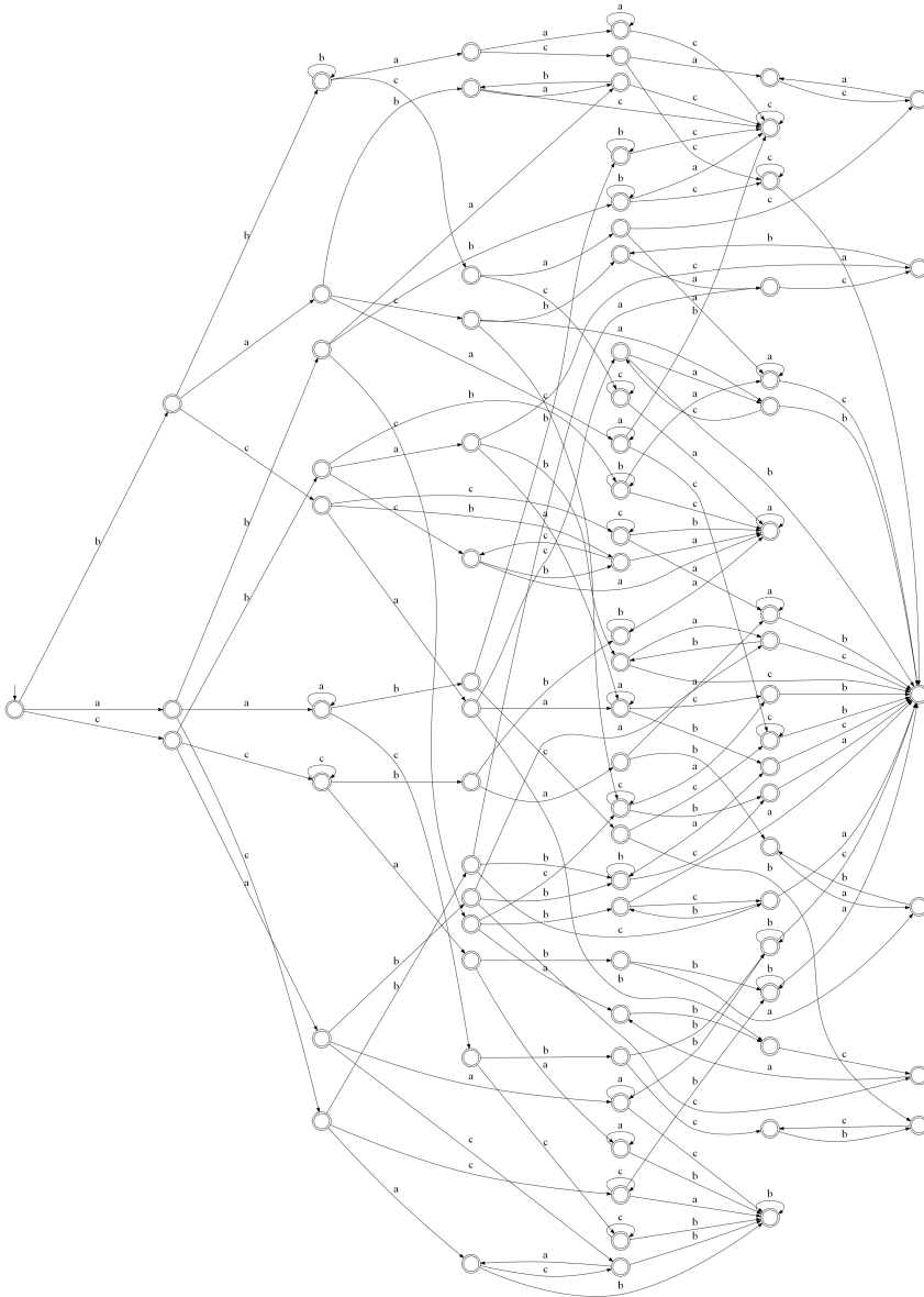
Figure 5.5: The minimal DFA recognizing L_{2,\{a,b,c\},\text{sing}} . [19, Figure 7].
