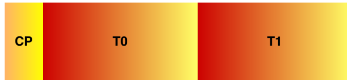
Figure 3.5: Representation of the preamble signal consisting of the CP and two consecutive training symbols: T0 and T1.
