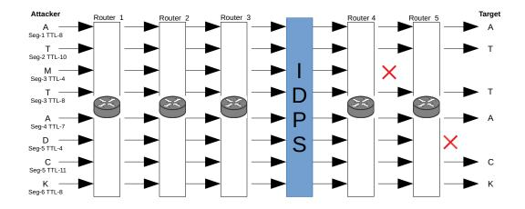
Figure 3.1: Attacking the target system with TTL Manipulation and Duplicate Insertion
