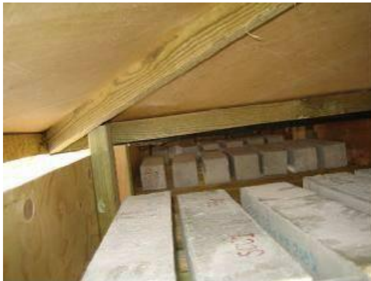
Figure 3.1. Sheltered concrete specimens for carbonation field test (Publication II).
