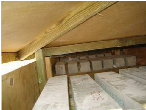
Fig. 4. Concrete specimen exposed to natural conditions at field.
