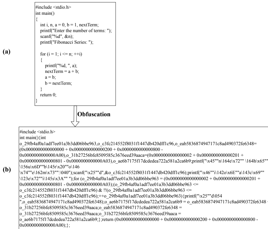
Figure 2.3: Excerpt from obfuscated piece of C code: a) original code, b) obfuscated version of the same code
