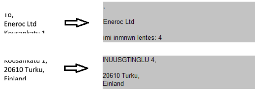
Figure 4.1: Example from an invoice that has been split to narrow image rows. These rows have then been processed with Tesseract OCR engine. The grey area shows how Tesseract has processed the whole lines correctly, but the split lines produce completely meaningless text.
