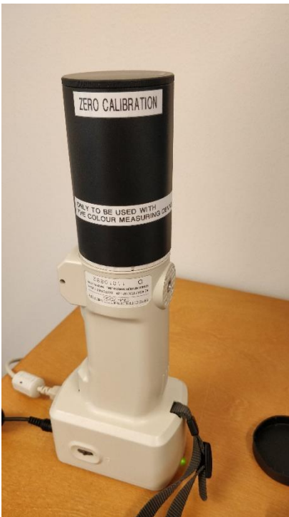
Figure 6. The Spectrophotometer used for measuring the samples optically.
