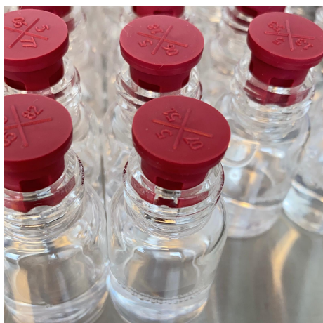
Figure 12. The cap of the bottles have little holes to make the evaporation of the liquid easier during freeze drying.
