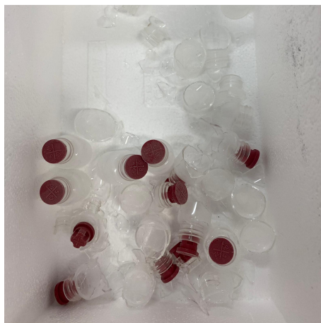
Figure 24. 32% of the freeze-drying bottles of GelMA broke at the -80^{\circ}\text{C} freezer.
