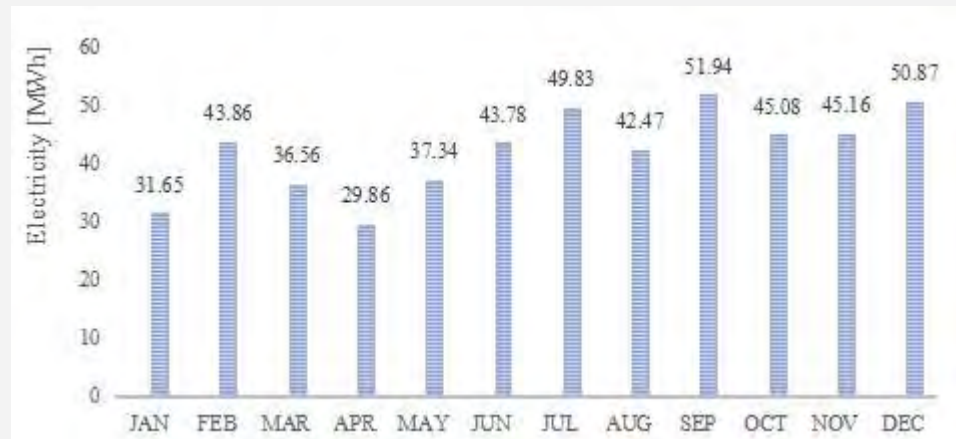
Figure 9. Electricity generation in a typical RoR Cuban SHP
