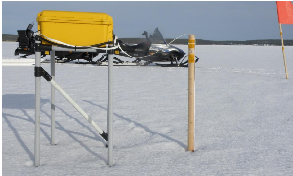
Figure 2. The updated SIMB deployment in lake Orajärvi, Sodankylä in 2013/2014 ice season. A wooden stick marked with scale is attached with thermistor string vertically distributed in along air-snow-ice-water. The SIMB is lifted with a fiberglass frame to ensure better iridium data transmission. (Photo by Jyrki Mattanen).
