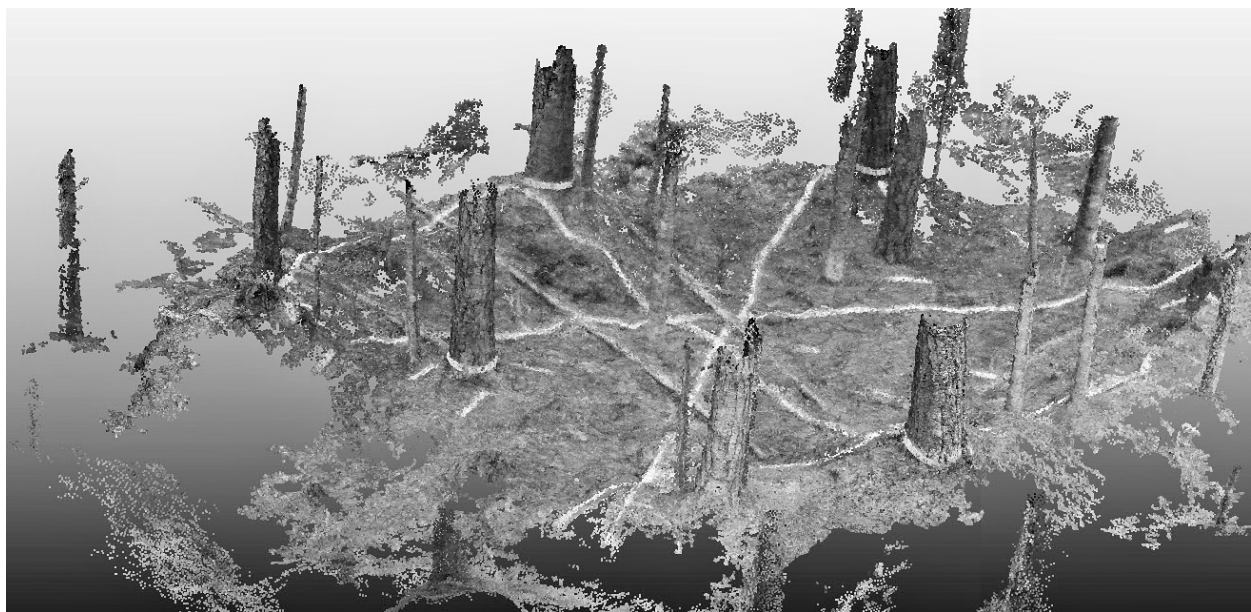
Figure 3: Example for a 3D reconstruction based on photography to assess microsite specific features of soil surface parameters in permanent sample plots. This technique can be used to assess differences in the soil surface heights (pits and mounds) or to measure distances or integrate aerial information.
