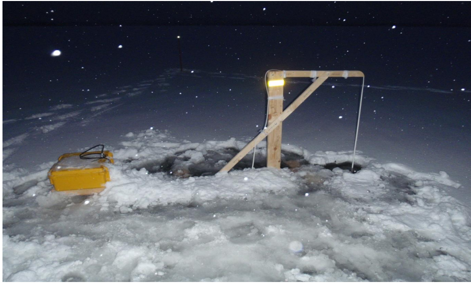
Figure 1. The initial deployment of SIMB in lake Orajärvi, Sodankylä in December 2011. A wooden frame is attached with thermistor string deployed vertically through the air-snow-ice and water. (Photo by Pekka Kosloff).
