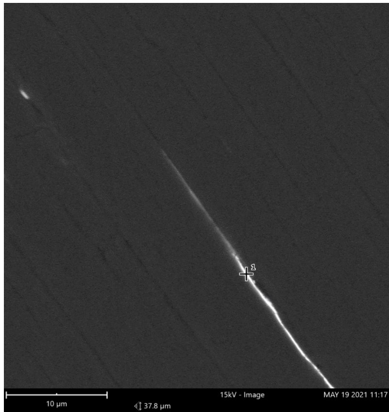
Figure 25. A backscattered electron microscope image of typical elongated inclusion inside a graphite grain. Spot analysis from the + mark showed elevated values of S, Fe, Si, and Al.
