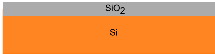
Figure 9. Schematic structure of the sample stack with \text{SiO}_2 layer on top of silicon substrate.
