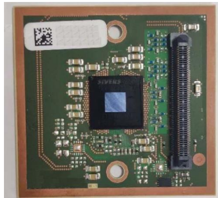
Figure 2-2: TRX BF06010 RF IC
