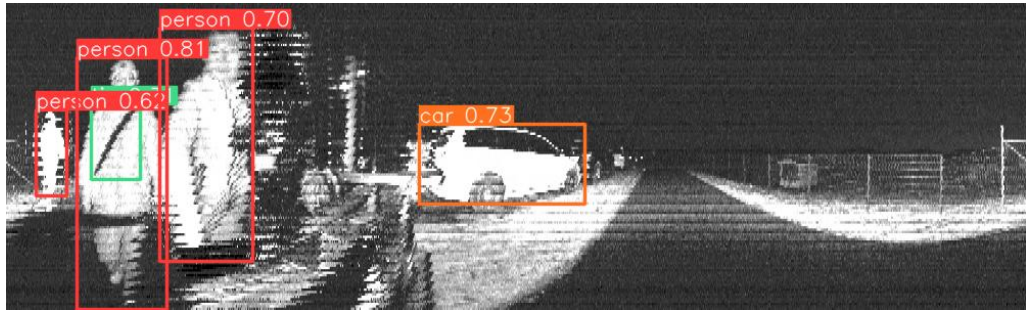
Figure 2.4: The results of running YOLOV5 on the signal images from the Ouster OS0-128.
