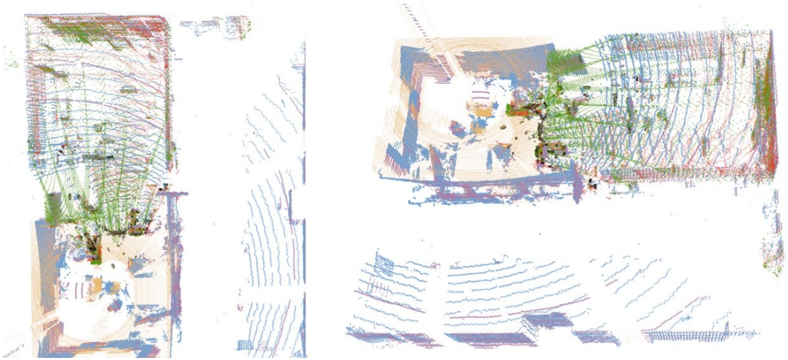
Figure 3.3: From an aerial perspective of the point cloud data assembled during the calibration of diverse LiDARs, the Livox Horizon and Avia are distinctly represented by shades of red and green. Concurrently, the VLP-16, OS1, OS0, and L515 sensors manifest themselves through point clouds colored in respective hues of purple, yellow, blue, and black.
