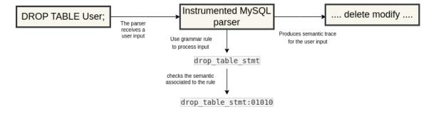
To achieve this objective we re-use the GAUR executable. It takes as input the Bison grammar to the instrument, the list of nonterminal-semantic pair, and a modified Bison skeleton. From these components, it will output an instrumented grammar file. This instrumented grammar file possesses a mapping of nonterminal towards their semantic, and function definitions to dynamically produce traces.
