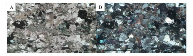
Figure 14. Microphotograph presenting chlorite vein in gabbro in the Tanhua mafic complex. A) PPL 5x, B) XPL 5x, both oxide gabbro sample U5212019R3 210.40 Abbreviations hbl – hornblende, pl – plagioclase, mg – magnetite, chl – chlorite and ti – titanite
