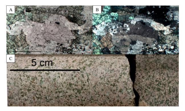
Figure 15. Microphotographs and photograph presenting general texture and presence of augite in gabbro in the Tanhua mafic complex. Sample U5212020R11 219.19 A) Microphotograph PPL 5x B) MicrophotographXPL 5x, C) Photograph of drill core. Abbreviations of A) and B) aug – augite, pl – plagioclase and qtz – quartz.
