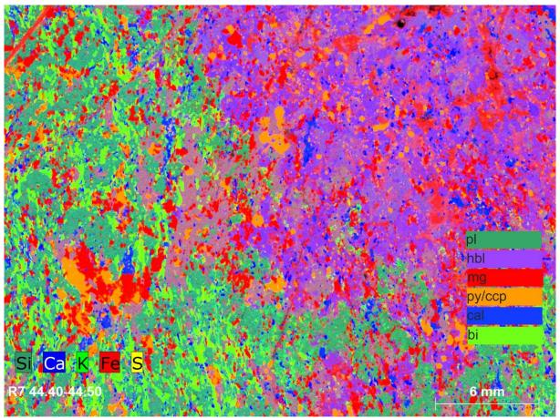
Figure 26. XRF-elementary maps presenting dissemination of magnetite in sample U5212019R7 44.40-44.50. The proposed minerals are based on common element content of minerals. Abbreviations pl – plagioclase, hbl – hornblende, mg –magnetite, py – pyrite, ccp – chalcopyrite, cal – calcite and bi – biotite.
