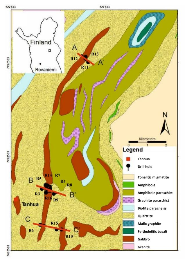
Figure 31. Geological map presenting the localization of three cross-sections (A – A' Kylälampi, B – B' Kannusvaara, C – C' Markkinaselkä) and drill hole of the Tanhua mafic complex. Coordinate system ETRS-TM35FIN. (Modified after DikiKP and Konnunaho et al. (2022)).
