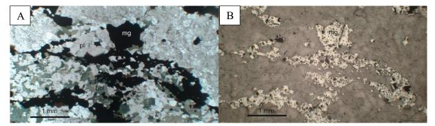
Figure 20. Microphotograph presenting occurrence of magnetite in diorite in the Tanhua mafic complex. Sample U5212019R3 277.15 A) PPL 2x, B) Reflected PPL 2x. Abbreviations hbl – hornblende, pl – plagioclase and mg – magnetite.
