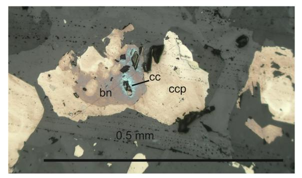
Figure 11. Microphotograph presenting occurrence of chalcopyrite, bornite and chalcocite in gabbros in the Tanhua mafic complex. The chalcocite has been altered to bornite which has been altered to chalcocite. Reflected PPL 20x gabbro sample U5212020R10 112.55. Abbreviations ccp – chalcopyrite, bn – bornite and cc – chalcocite.
