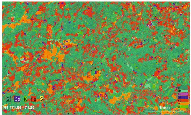
Figure 29. XRF-elementary maps of sample U5212019R5 171.05.171.20 presenting tonalite in the Tanhua mafic complex. The proposed minerals are based on common element content of minerals. Abbreviations pl – plagioclase, hbl – hornblende, mg –magnetite, py – pyrite, qtz – quartz, cal – calcite and bi – biotite.
