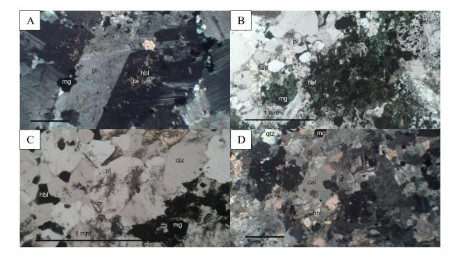
Figure 22. Microphotograph presenting A) poikilitic texture and albite twinning of plagioclase, sample U5212019R4 65.45 XPL 2x B) Magnetite overprint on hornblende, sample U5212019R3 330.35 PPL 5x, C) Occurrence of zircon, sample U5212019R3 330.35 PPL 10x D) Occurrence of calcite in tonalite in the Tanhua mafic complex, sample U5212019R3 330.35 XPL, 2x. Abbreviations hbl – hornblende, pl – plagioclase, bi – biotite, mg – magnetite scp – scapolite, qtz –quartz, zr– zircon and cal – calcite.
