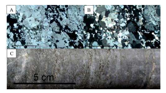
Figure 19. Microphotographs and photograph presentinggeneral texture of diorite in the Tanhua mafic complex. Sample U5212019R7 56.85 A) Microphotograph PPL 5x, B) Microphotograph XPL 5x. C) Photograph of drill core. Abbreviations of A) and B) hbl – hornblende, pl – plagioclase mg – magnetite and bi – biotite.
