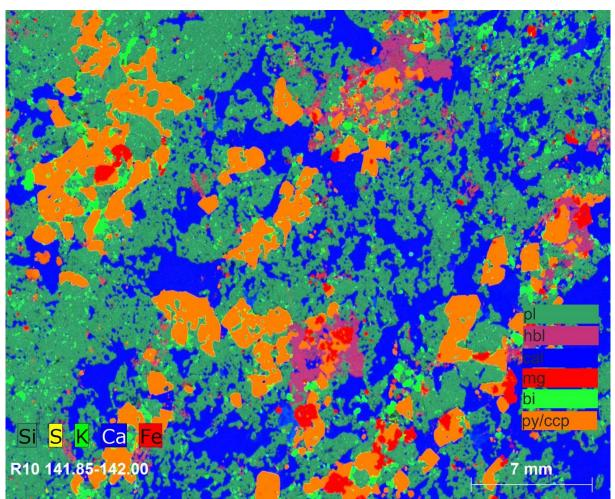
Figure 27. XRF-elementary maps of sample U5212020R10 141.85-142.00 presenting calcium alteration of the Tanhua mafic complex. The proposed minerals are based on common element content of minerals. Abbreviations pl – plagioclase, hbl – hornblende, mg –magnetite, py – pyrite, ccp – chalcopyrite, cal – calcite and bi – biotite.
