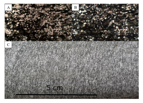
Figure 24. Microphotograph presenting general texture and grain size of mafic vulcanic rock in the Tanhua mafic complex. A) PPL 2x, B) XPL 5x. Sample U5212019R14 84.50 C. Photograph of drill core near of the sample U5212019R14 84.50 presenting vulcanic rock in the Tanhua mafic complex. Abbreviations of A) and B) hbl – hornblende, pl – plagioclase and mg – magnetite.
