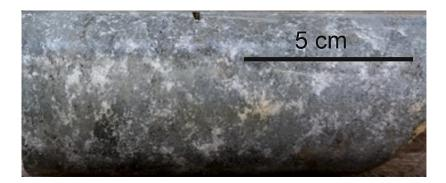
Figure 16. Photograph of drill core near of the sample U5212019R6 131.35 presenting remained mottled gabbro.
