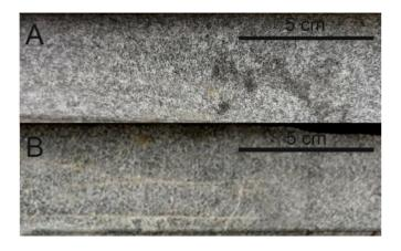
Figure 6. Photograph of drill core from the Tanhua mafic complex. A) Gabbro sample U5212019R14 64.30, B) Oxide gabbro sample U5212020R16 41.40
