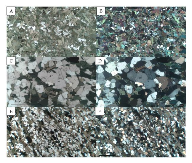
Figure 7. Microphotograph presenting general texture and grain size of gabbro in the Tanhua mafic complex. A) and B) Sample U5212019R13 159.80, A) PPL 5x. B) XPL 5x and D) sample U521019R14 22.20 C) PPL 5x, D) XPL 5x. E) and F) gabbro sample U5212019R6 176.30, E) PPL 2x, F) XPL 2x. Abbreviations hbl – hornblende, pl – plagioclase, bi – biotite and mg – magnetite.
