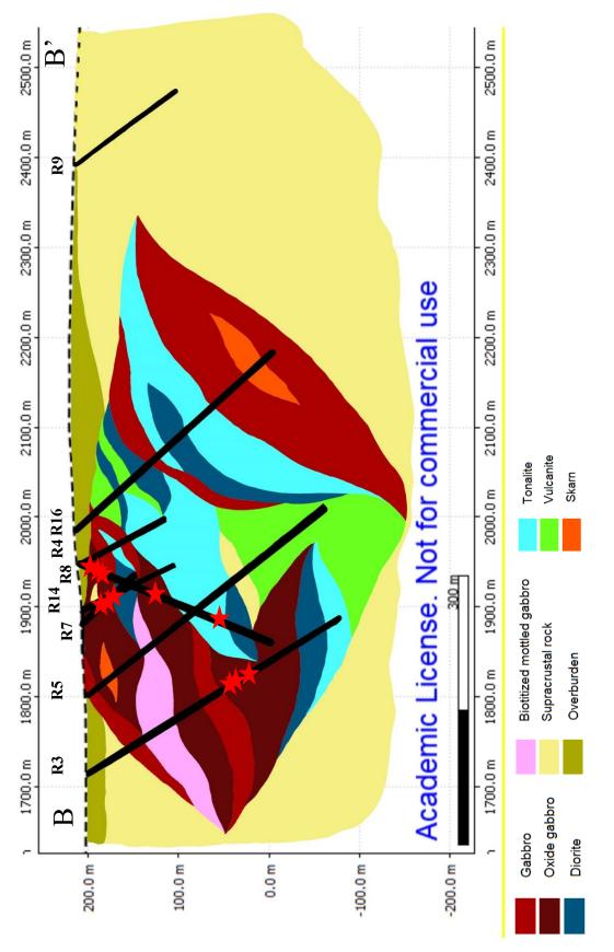
Figure 33. Simplified cross section of Kannusvaara. Red stars symbolize the most significant mineralizations in the Tanhua mafic complex after Konnunaho et al. (2022).
