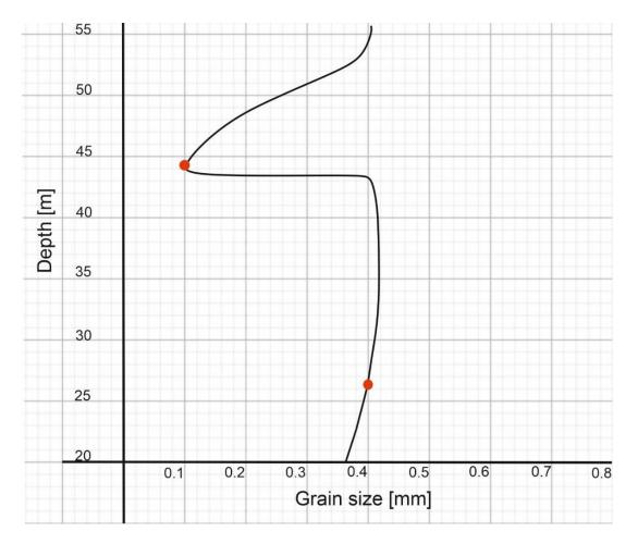
Figure 30. A draft presenting the estimated change of the grain size in drill core U5212019R8 between depths 20m and 55m. The red dots are measured points confirmed with thin sections. The black line is the estimated grain size along the drill core.
