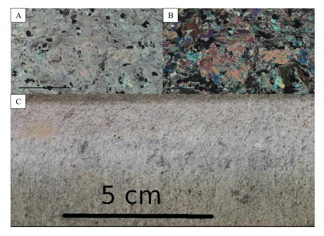
Figure 23. Microphotograph presenting general texture of peridotite in the Tanhua mafic complex. A) PPL 5x, B) XPL 5x. Sample U5212019R13 82.35, C) Photograph of drill core near of the sample U5212019R13 149.05 presenting pyroxene in the Tanhua mafic complex. Abbreviations of A) and B) amp – amphibole and mg – magnetite.
