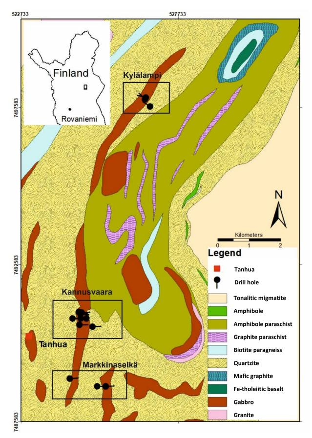
Figure 5. Geological map from the area of the Tanhua mafic complex. Coordinate system ETRS-TM35FIN (Modified after DigiKP and Konnunaho et al. (2022))
