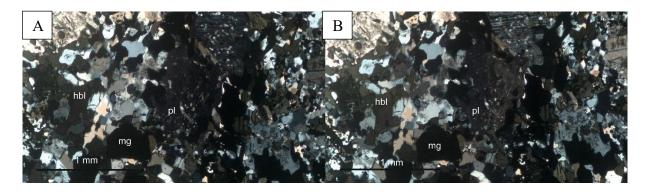
Figure 9. Microphotograph presenting poikilitic and zoned texture in gabbros in the Tanhua mafic complex. A) and B) XPL 5x gabbro sample U5212019R14 64.30. Abbreviations hbl – hornblende, pl – plagioclase and mg – magnetite.
