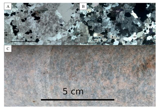
Figure 21. Microphotographs and photograph presenting general texture of tonalite in the Tanhua mafic complex. Sample U5212019R7 120.70 A) Microphotograph PPL 5x, B) Microphotograph XPL 5x. C) Photograph of drill core. Abbreviations of A) and B) hbl – hornblende, pl – plagioclase, mg – magnetite and qtz – quartz.
