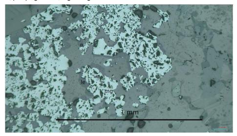
Figure 13. Microphotograph presenting alteration of magnetite to leucoxene. Biotitized mottled gabbro Sample U5212019R3 253.20. Reflected 10x. Abbreviations mg – magnetite, le – leucoxene.
