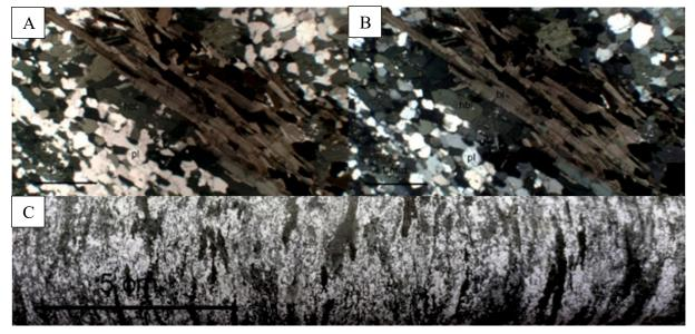
Figure 18. Microphotographs and photograph presenting general texture of biotitized mottled gabbro in the Tanhua mafic complex. A) PPL 2x, B) XPL 2x. Sample U5212019R5 83.30 C) Photograph of drill core sample U5212019R3 95.45. Abbreviations of A) and B) hbl – hornblende, pl – plagioclase and bi – biotite.
