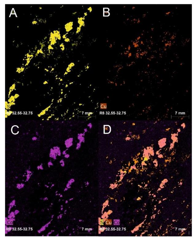
Figure 25. XRF elementary maps of sample U5212019R8 32.55-32.75 presenting the occurrence of pyrite and chalcopyrite. In addition, present the occurrence of Co in pyrite. A) sulphur presented, B) copper presented, C) cobalt presented, D) sulphur, copper and cobalt presented together.
