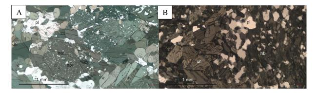
Figure 8. Microphotograph presenting A) exsolution texture of quartz in hornblende PPL 5x gabbro sample U5212020R16 298.40. B) uralite in the Tanhua mafic complex. PPL 5x remained mottled sample U5212019R6 131.35. Abbreviations hbl – hornblende, pl – plagioclase, qtz – quartz and ur – uralite.
