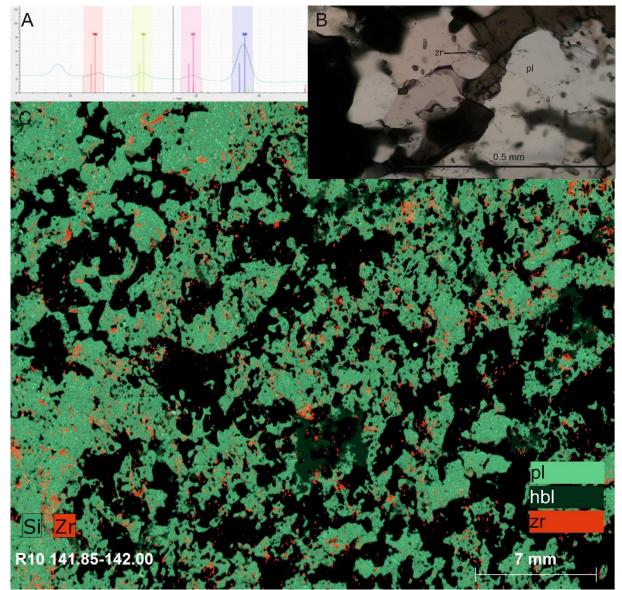
Figure 28. Sample U5212020R10 141.85-142.00 A) XRF spectrum of zirconium. B) Microphotograph of occurrence of zircon together within plagioclase PPL 20x C) XRF-elementary map presenting the location of zircon. The proposed minerals are based on common element content of minerals. abbreviations pl – plagioclase, hbl – hornblende and zr – zircon.
