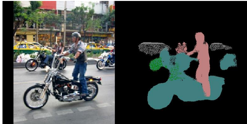
Figure 4.8: Horizontal Partitioning Semantic Segmentation Bad Merge Results Example
