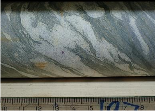
Figure 16. Drill core ISO17609 (Kati area) with foliation parallel shearing of calcite (type 4) vein and mafic tuff. Drill core was not oriented.
