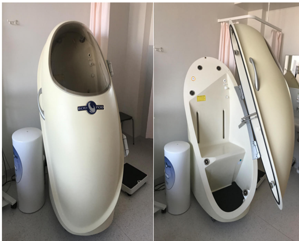
Figure 7. Air displacement plethysmography (the Bod Pod system, COSMED, Inc., Concord, CA, USA) with predicted thoracic gas volume was used to estimate body composition.
