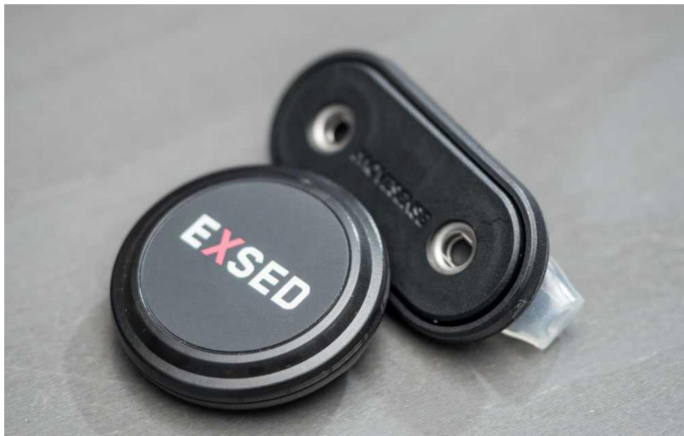
Figure 5. A visual presentation of the hip-worn tri-axial accelerometer used throughout the six-month intervention period (ExSed Movesense, Suunto, Vantaa, Finland).
