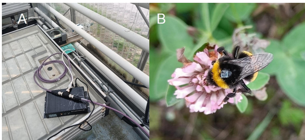
Figure 3. (A) Radio frequency identification device: Controller (ID ® BEEcontroller) attached to a reader placed on top of the entrance tunnel. (B) A bumblebee tagged with an RFID tag with a unique identification number.
