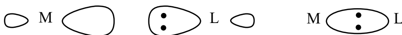
Figure 3. Metal ion's empty hybrid atomic orbital and the ligand's lone electron pair in a hybrid atomic orbital result in a coordinate covalent bond. Figure based on ref 36. 36
