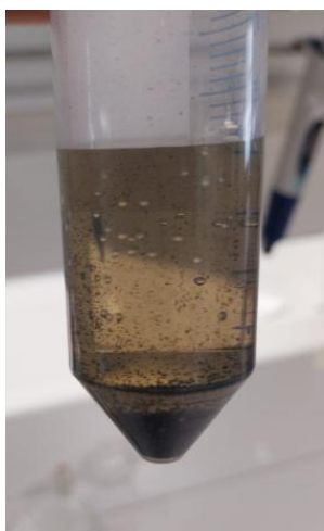
Figure 14. Partially reduced H4 sample with some black particles.
