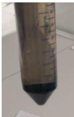
Figure 16. After chemical reduction, all rGO particles settle at the bottom.
