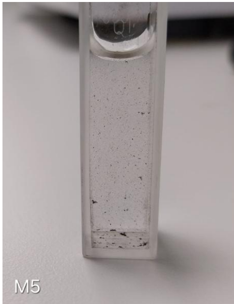
Figure 19. Consistency of sample M5 with visible larger clumps of rGO.
