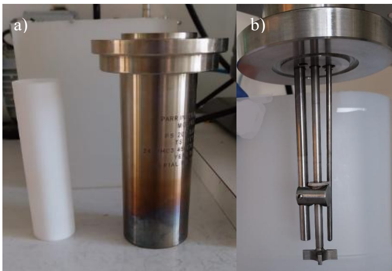
Figure 5. a) The Teflon liner and reactor chamber b) The sampling tube, stir bar and temperature probe.
