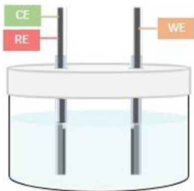
Figure 11. Schematic of the 2-electrode symmetric electrochemical set up using grafoil electrodes with the WE, CE and RE placements shown.
