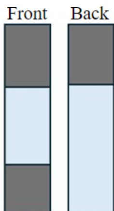
Figure 7. Schematic of the electrodes with the tape placement in blue.
