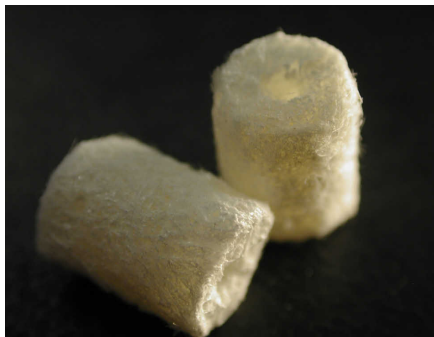
Figure 7. FRC implants with porous surface for segment defect construction in study IV ( \varnothing = 8.3 mm, l = 10 mm, intramedullar canal \varnothing = 3 mm).
