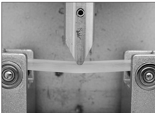
Figure 10. Test setup for the three point bending test.
