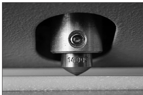
Figure 11. Test setup for Vickers surface microhardness test.
