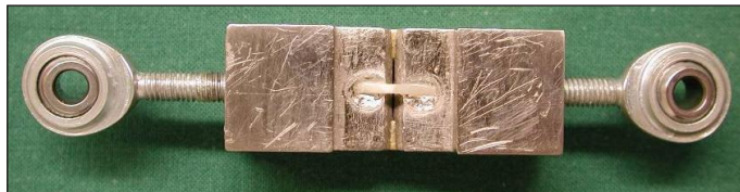
Figure 13. Test jig for microtensile measurement.
