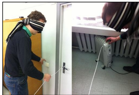
Fig. 7. A guide wire system to mimic the navigational capabilities of real blind person.
