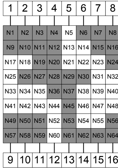
Figure 6.7: A fragmented situation with 36 cores occupied (gray), and 28 cores free (white).
