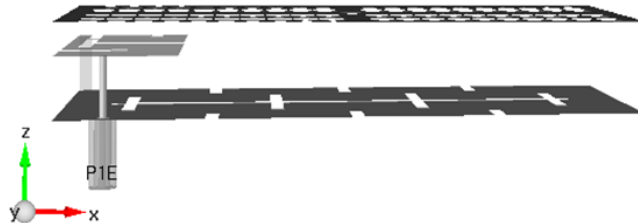
Figure 3.1: Side view of antenna with slotted plane and with EBG Structure
