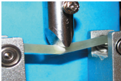
Figure 1 Three-point bending test of fiber-reinforced composite (FRC) cylinder demonstrating high bending strength and toughness with delamination of individual fibers from the polymer matrix at the point of final failure (white region). The unidirectional E-glass fibers maintain the structural integrity of the FRC cylinder after failure.
