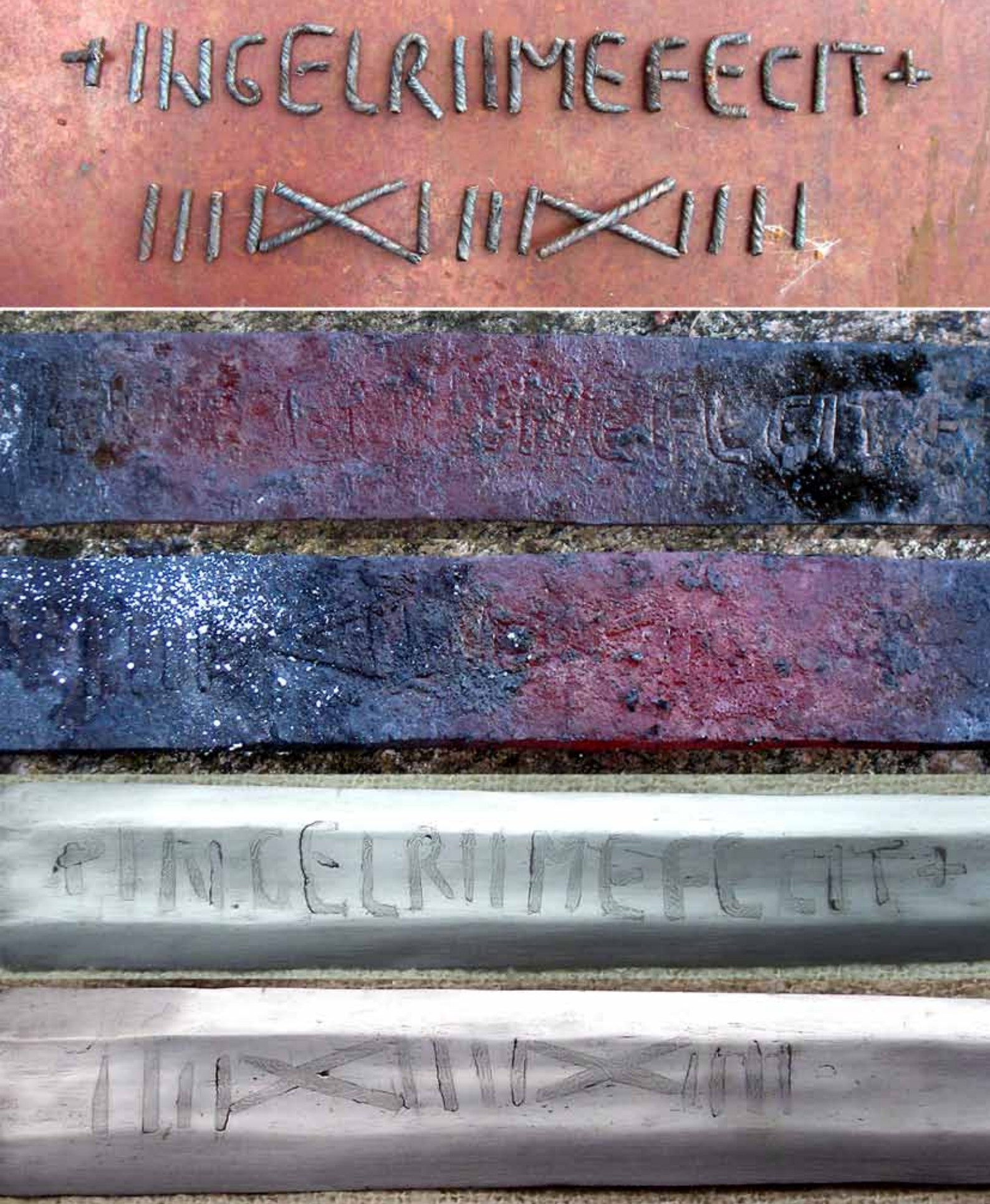
Figure 83. The stages of the eleventh experiment: 1. Letters and marks formed from pattern-welded rods, 2. The same inlays welded into a blade blank. The inlays have not been considerably flattened, but only sunk into the blade, 3. A completed, polished and etched blade.
