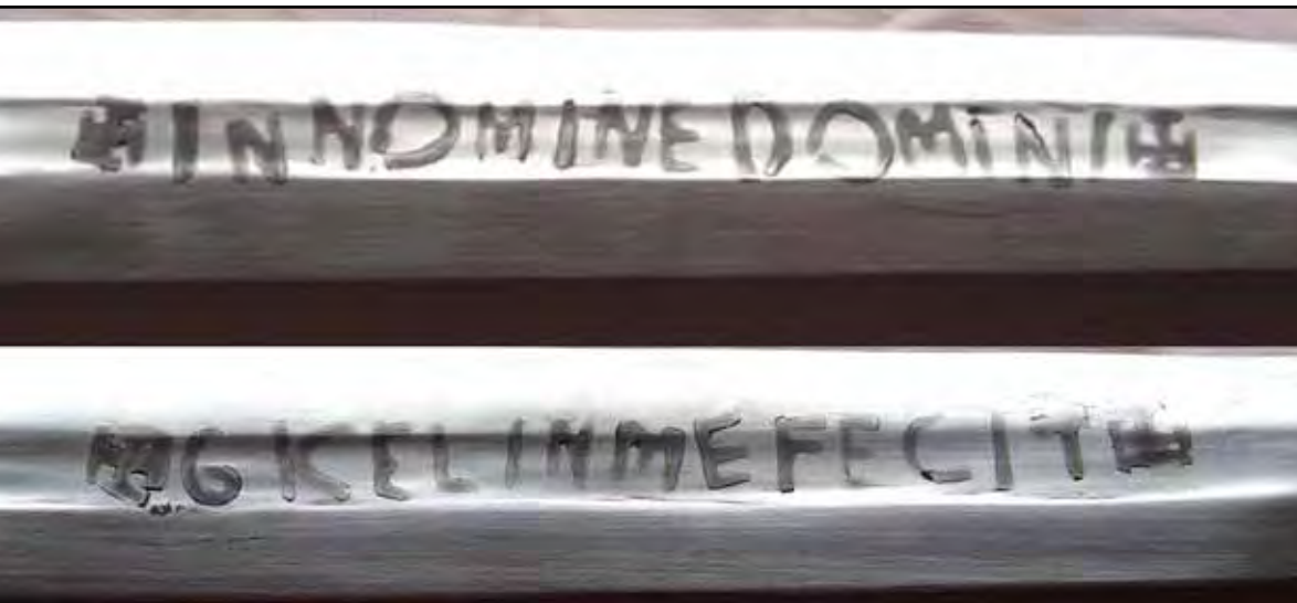
Figure 84. The thirteenth experiment. The blade is polished and etched to show the steel inlays.
