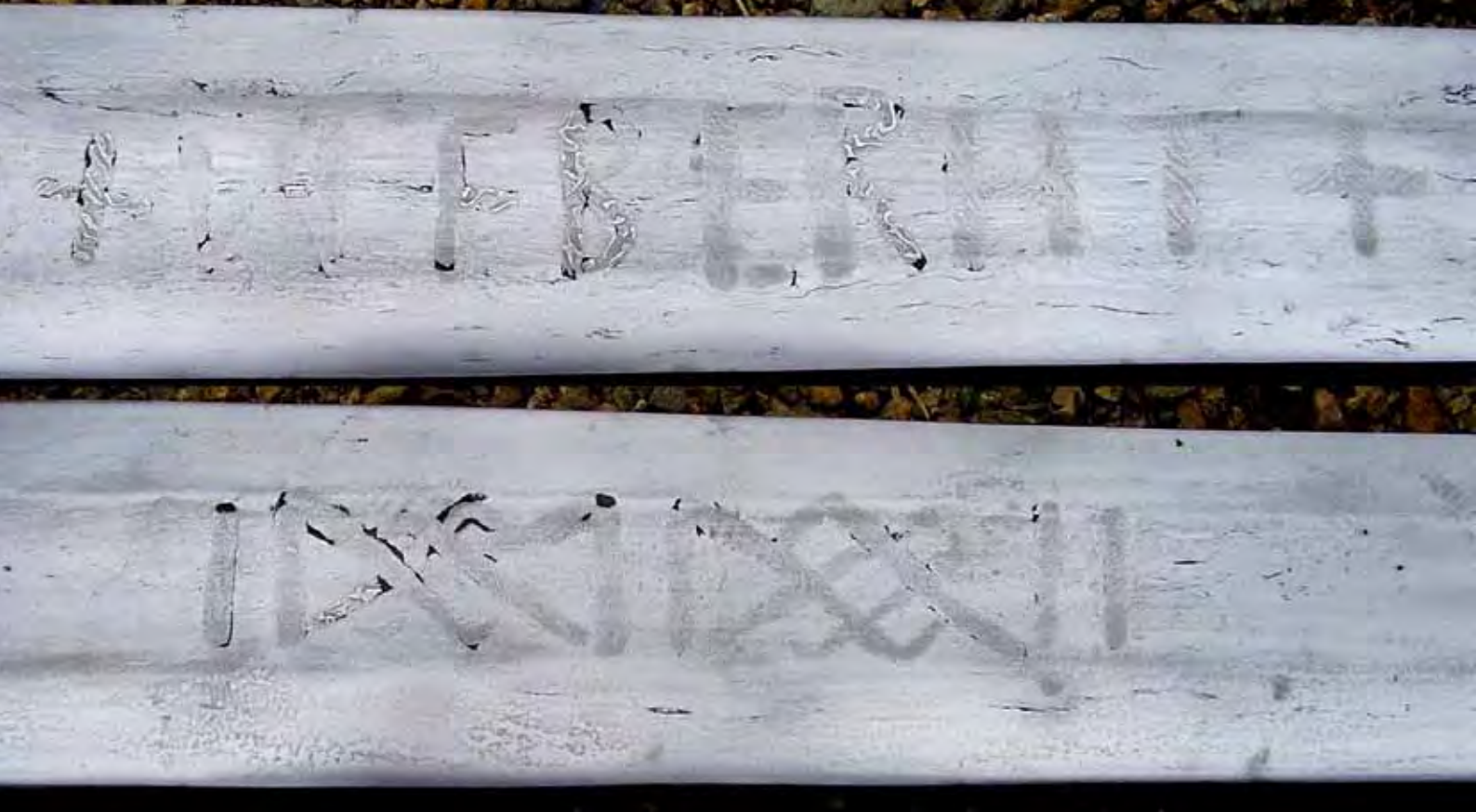
Figure 82. A finished, polished and etched blade showing pattern-welded inlays and the fibrous, longitudinal structure of the steel produced in the tenth experiment.
