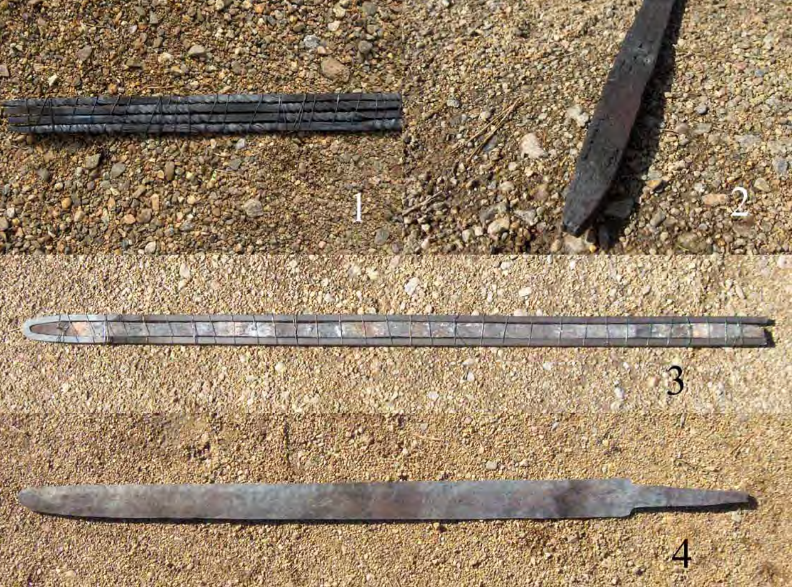
Figure 76. Example of the stages of forge-welding a pattern-welded blade to one piece: 1. Four partially twisted rods tied together with thin iron wire, 2. Twisted rods welded together, 3. The steel for the cutting edges tied to the pattern-welded core, 4. The completely welded blade which has been hand-forged to sword shape.
