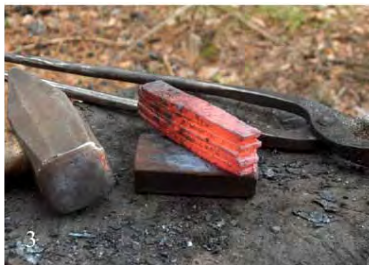
Figure 78. The making of a pattern-welded pack: 1. A pack made from alternating sheets of iron and steel, bound together with iron wire, 2. Forge-welding the pack by hammering, 3. A completely welded and solid pack.
