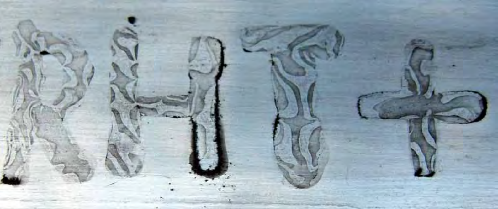
Figure 80. Close-up view of the inlaid letters of the seventh experiment. The lower right tip of the letter H has not been properly welded, but the letter still remains intact in the blade.
