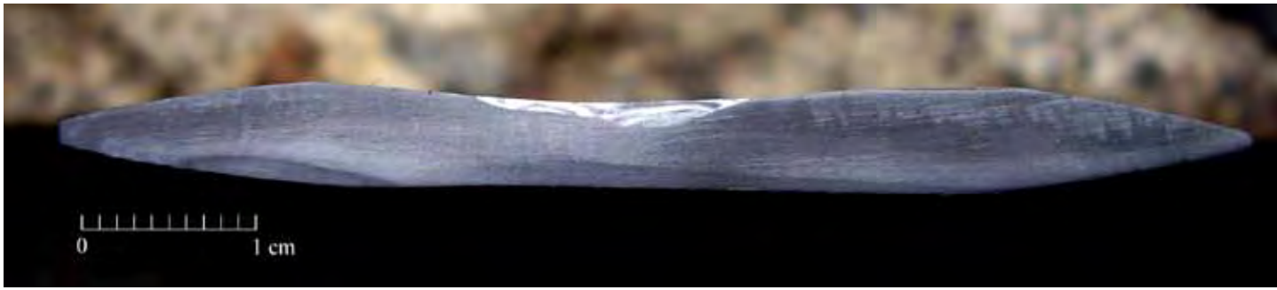
Figure 81. The polished and etched cross-section of the blade made in the ninth experiment. The carbon steel blade has become etched dark grey, while the inlays are visible as darker and brighter lines at the top surface of the cut blade. The cut inlay, the cross, sank ca. 1.4 millimetres in its centre, while a single inlaid rod sank about 0.7 millimetres.
