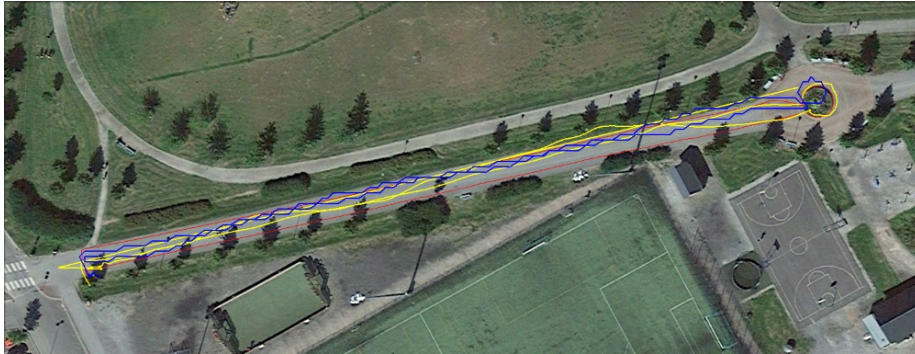
Figure 8: Mobile measurements for Apple iPad 3. The red line is the reference route, the yellow line is the native application measurement and the blue line is the Unity3D measurement with one meter step.
