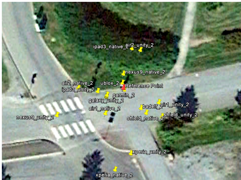
Figure 7: Average positions reported by the measured devices and the location of the reference point (the red pin) during static measurement 2.
