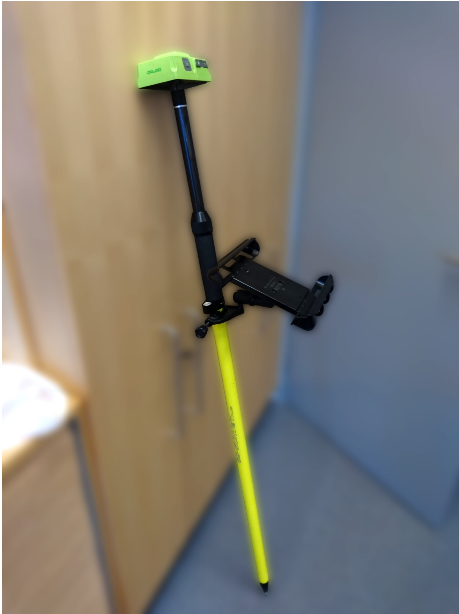
Figure 2: Javad Triumph-2 and the tablet grip that were used in the mobile measurements.
