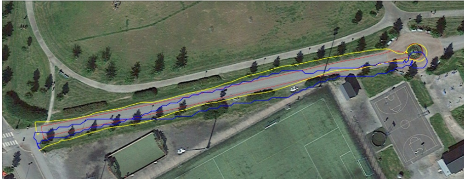
Figure 11: Mobile measurements for Sony Xperia Z4 Tablet. The red line is the reference route, the yellow line is the native application measurement and the blue line is the Unity3D measurement with one meter step.
