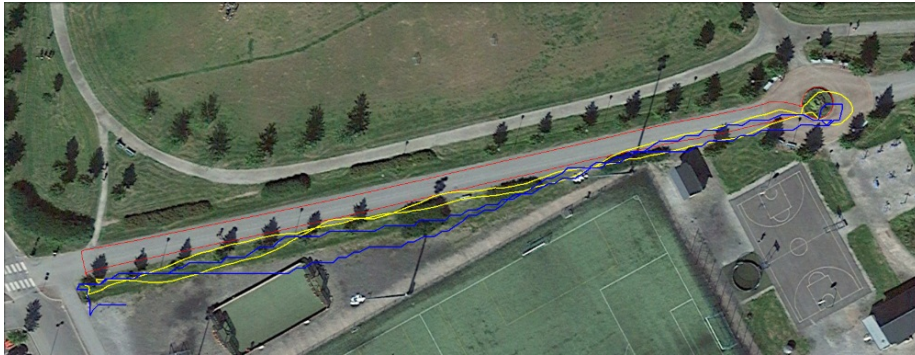
Figure 12: Mobile measurements for Samsung Galaxy Tab S2. The red line is the reference route, the yellow line is the native application measurement and the blue line is the Unity3D measurement with one meter step.
