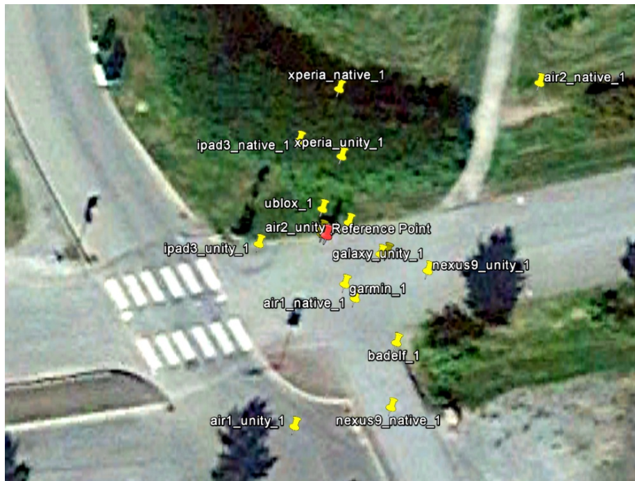
Figure 6: Average positions reported by the measured devices and the location of the reference point (the red pin) during static measurement 1.
