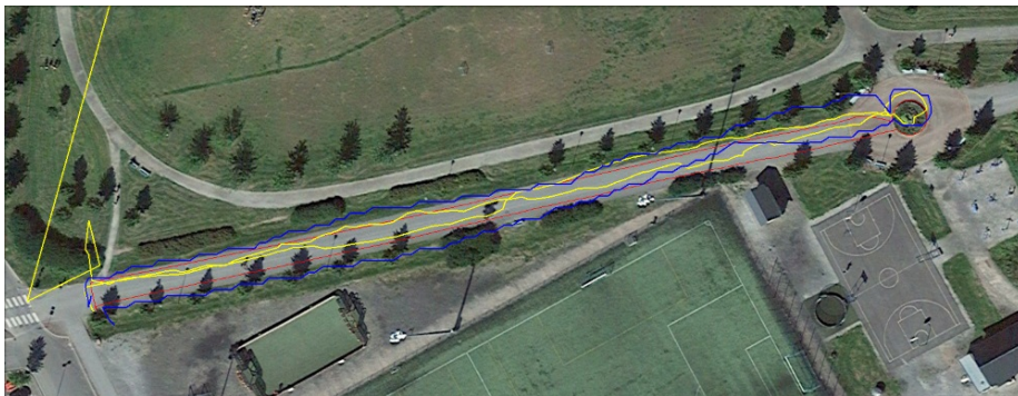
Figure 10: Mobile measurements for Apple iPad Air 2. The red line is the reference route, the yellow line is the native application measurement and the blue line is the Unity3D measurement with one meter step.
