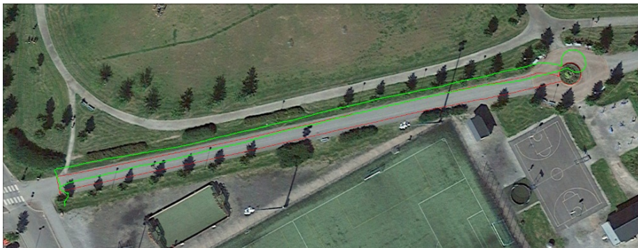
Figure 16: Mobile measurements for Garmin GLO. The red line is the reference route, the yellow line is the native application measurement and the blue line is the Unity3D measurement with one meter step.
