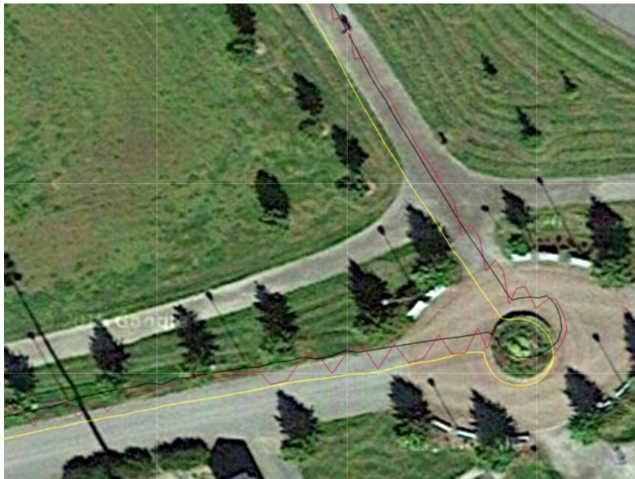
Figure 4: An image representing the effect of an RTK-GPS correction signal. The yellow line depicts Javad Triumph-2 with a working correction signal, the black line depicts the same device without a correction signal, and the red line depicts again the same device but with a bad signal quality. The red line can be seen bouncing between corrected and erroneous coordinates.
