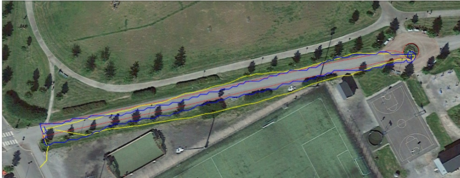
Figure 14: Mobile measurements for HTC Nexus 9. The red line is the reference route, the yellow line is the native application measurement and the blue line is the Unity3D measurement with one meter step.
