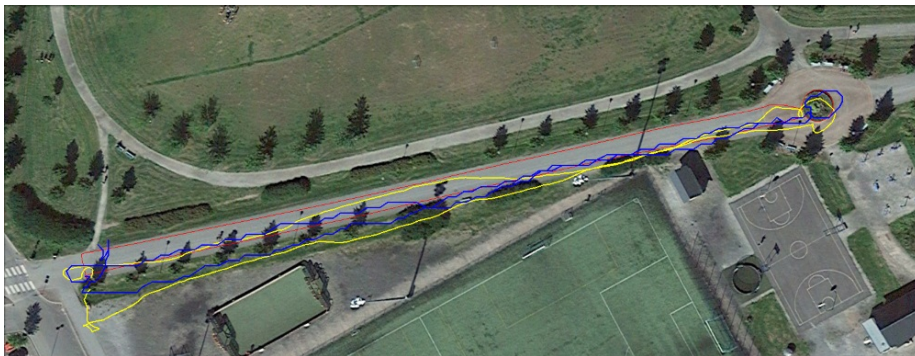
Figure 13: Mobile measurements for NVIDIA SHIELD Tablet. The red line is the reference route, the yellow line is the native application measurement and the blue line is the Unity3D measurement with one meter step.
