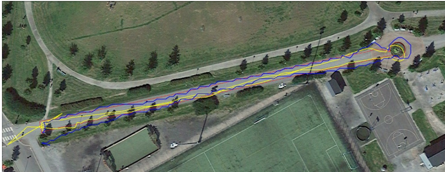
Figure 9: Mobile measurements for Apple iPad Air. The red line is the reference route, the yellow line is the native application measurement and the blue line is the Unity3D measurement with one meter step.
