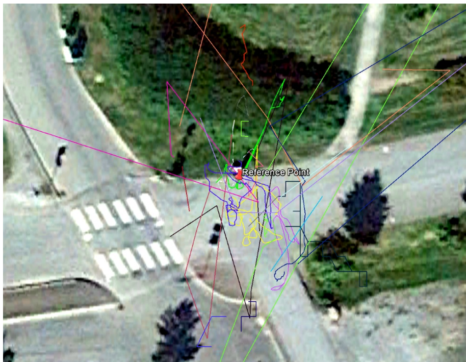
Figure 5: Lines drawn of each static measurement. The "wandering" lines clearly show how each device reported varying coordinates during the measurements.
