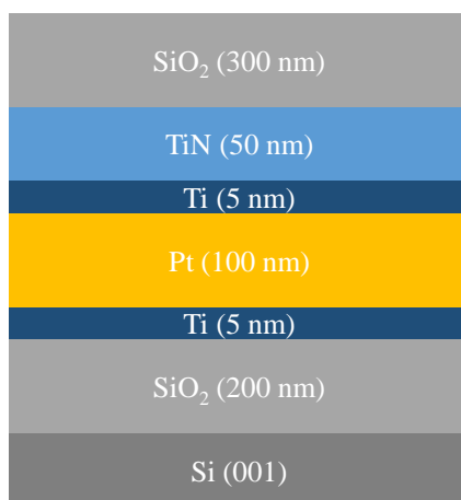
Figure 5.1: Sample after deposition of bottom electrode materials.
