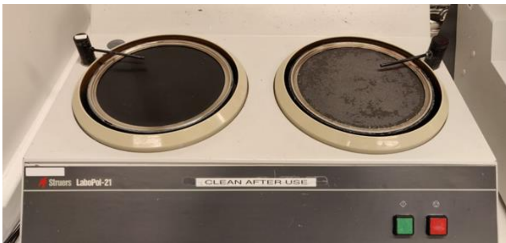
Figure 2. FRC posts and PMMA blocks were ground with Struers LaboPol-21.
