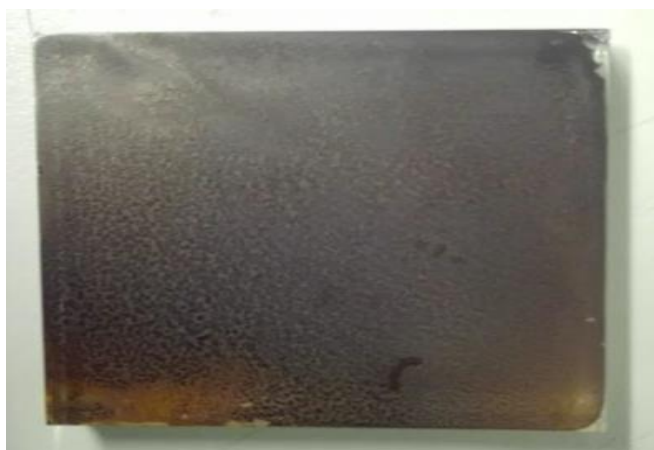
Figure 21: Spin coated perovskite on top of FTO substrate after annealing process
