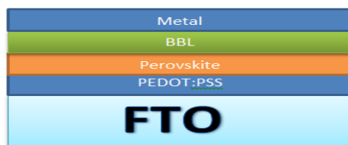
Figure 9: Basic framework of solar cell using perovskite
