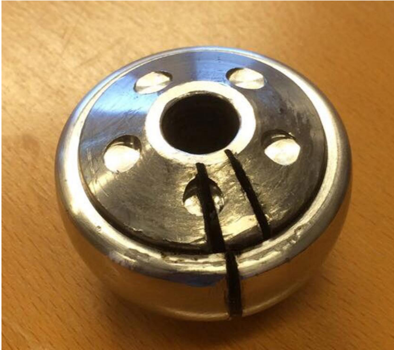
Figure 12. M2a-Magnum head after difficult removal
