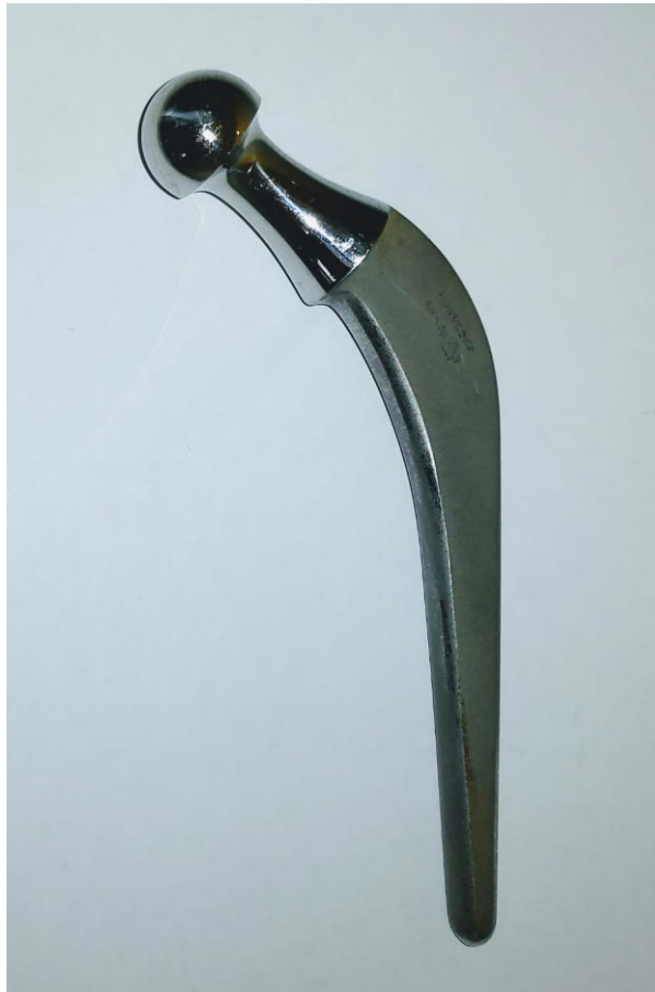
Figure 3. Stem of Charnley's hip arthroplasty.
