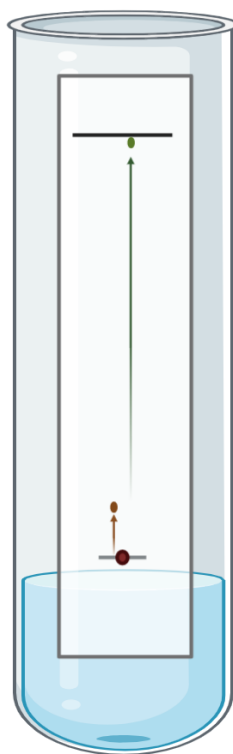
Figure 4. Visualization of compound separation on iTLC strip. The solute is placed as a small dot on the line drawn. The strip is placed in the development chamber, where the developer is pooled below the line containing the solute. As the developer moves up the strip's capillary network, the components within the solute are separated based on various properties depending on the conditions used. In this example, the strip has silica gel coating and the developer is a slightly acidic buffer. As the buffer travels up the network, the most polar substance binds first to the silica in the coating, therefore traveling to the solvent front, shown as the black line at the top of the strip, first. The less polar compound remains at the bottom of the strip, as most of the silica gel has already been bound. Created on Biorender.com.
