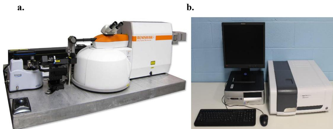
**Figure 3.3 Image of (a) Raman spectrometer from Renishaw and (b) UV-vis spectrometer from Agilent Cary 60. [61].**
