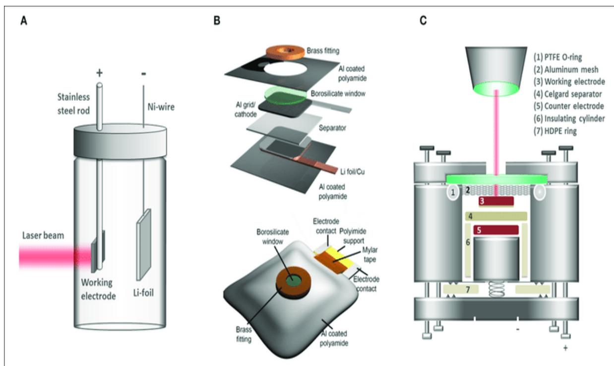
**Figure 2.4** Typical cell designs for in situ/operando Raman spectroscopy. (A) Beaker (pyrex) cell design used e.g., by Inaba et al. (1995). (B) Pouch cell from Ghanty et al. [reprinted from reference (Ghanty et al., 2015) with permission of John Wiley and Sons]. (C) Custom-made coin-cell type design developed in our group [37].
