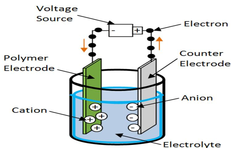
Figure 2.3 Illustration of two electrode electrolytic cell and its components [32].
