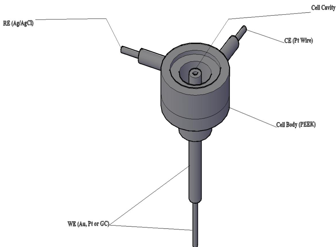
Figure 3.1 (a) Picture of Raman cell setup and (b) Schematic diagram of Raman cell showing all parts.
