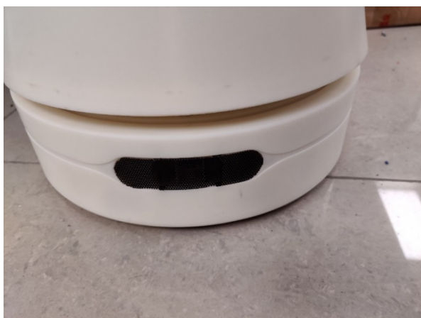
Figure 2-21 The place where the ultrasonic sensor is installed.
