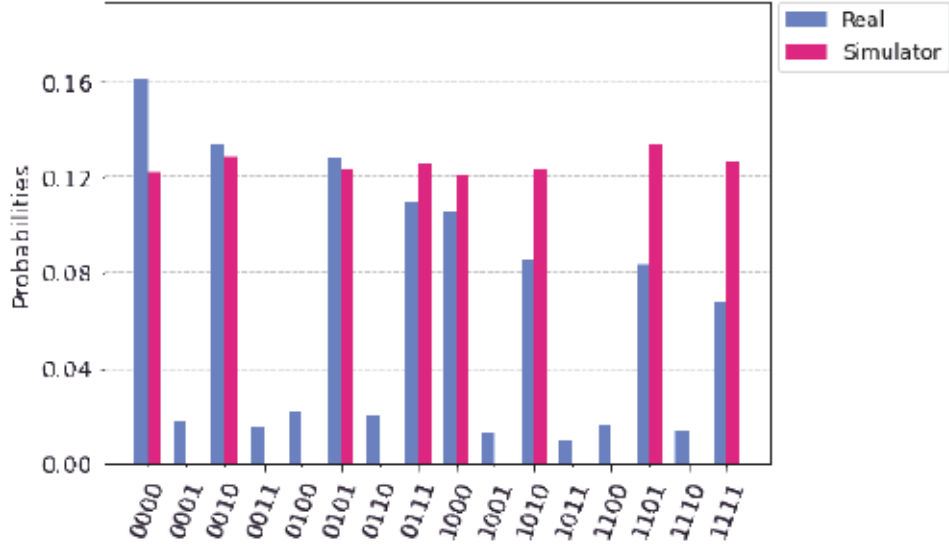
Figure 13: The results of two-to-one experiment comparing the simulation to the results from the real quantum computer, with 8192 shots on each.
