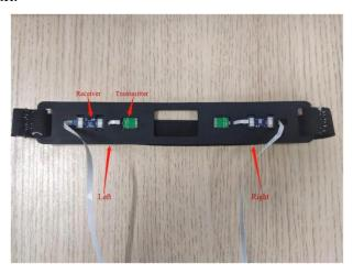
Figure 2.5 NIRS signal collection model
