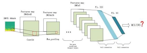
Figure 3.9 CNN + STFT model
