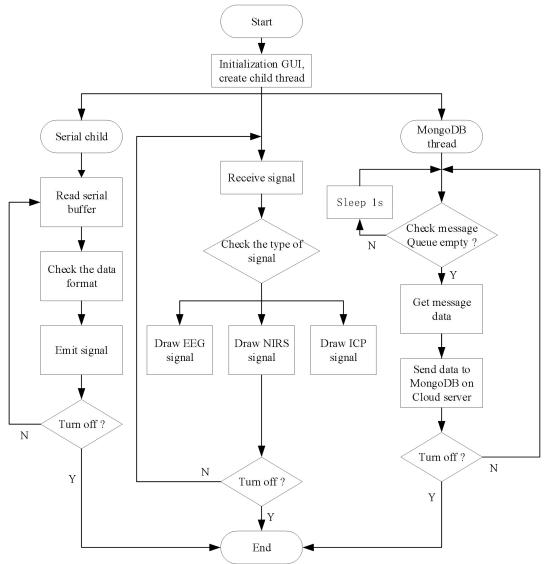
Figure 5.3 The workflow of GUI
