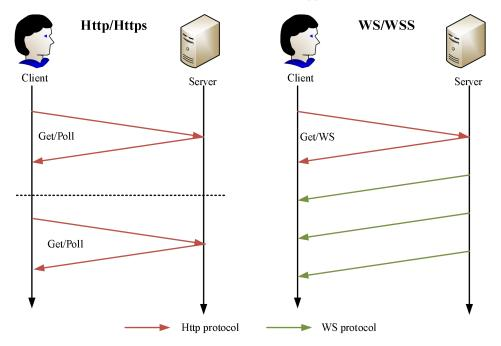
Figure 5.7 Communication based on Http and WebSocket protocol
