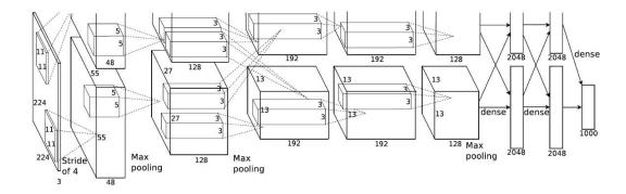
Figure 2.8 AlexNet structure [60]
