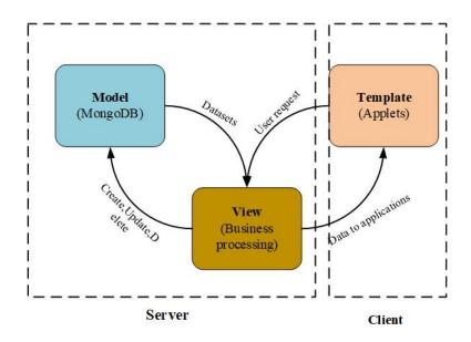
Figure 5.5 The structure of Django (MTV)
