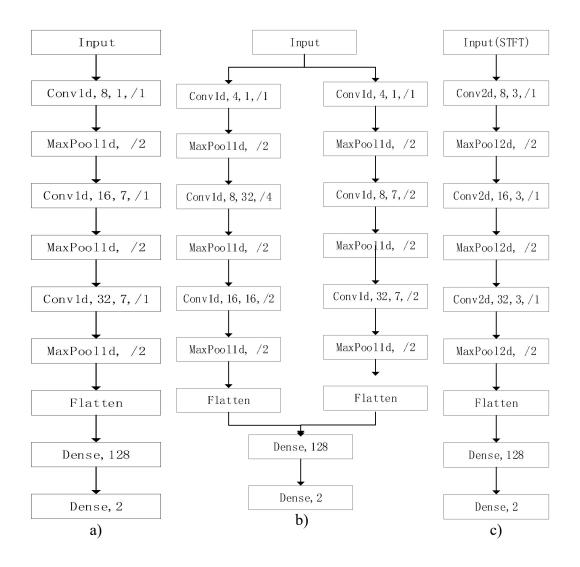
Figure 4.5 (a): normal 1D CNN model with 3 convolutional layers and 2 fully connected layers. (b): model with using different size of kernels in convolutional layers, and combine the features after Flatten. (c): the same frame with (a), the difference is using 2D convolutional kernels in 2D time-frequency domain images from STFT.
