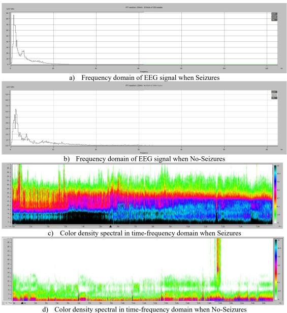
Figure 4.4 Frequency characteristics of EEG signal from Huashan Hospital dataset
