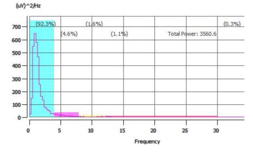
Figure 3.3 EEG sample signal from a person with nominal neural conditions.
