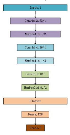
Figure 3.4 1D-CNN Network
