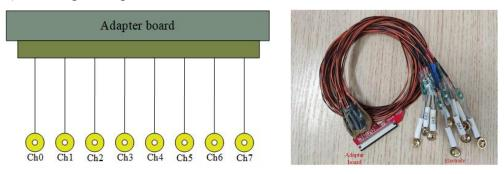
Figure 2.3 EEG Electrode Structure
