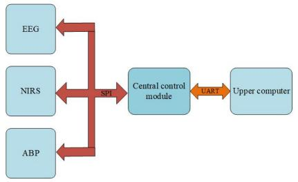
Figure 2.1 Hardware system structure
