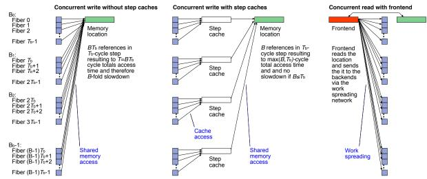
Figure 3. Concurrent in the baseline system (with no step caches), concurrent write with step caches and concurrent read with a the fronend.
