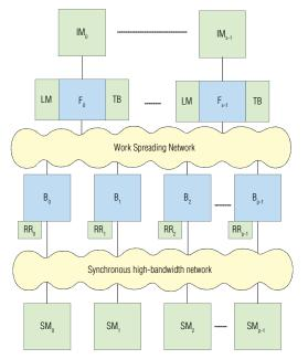
Figure 2. The overall structure of TPA (IM=instruction memory, F=processor frontend, LM=local memory, TB=TCF buffer, B=processor backend unit, RR=replicated register block, SM=shared memory module). The external memory system is not shown.
