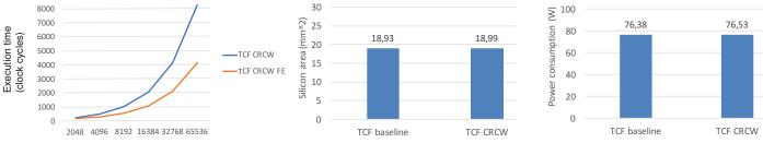
Figure 5. The differences in execution time of the spread benchmark implemented with the backend only access technique and frontend access technique (left), the silicon area (middle) and power consumption estimates (right) for 11 nm silicon process.
