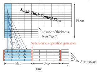
Figure 1. A thick control flow, change of thickness from 16 to 11 and execution as steps. A step of execution in a TCF-aware processor. The machinery assignings T=16 fibers for execution in P=4 processors and guarantees synchronicity between the steps.
